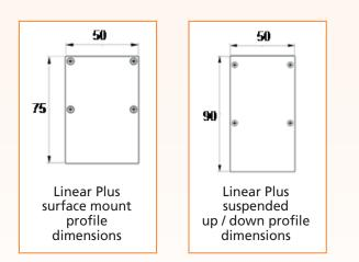
Standard Lengths Opal / Microprism 1145mm / 1425mm Dark Light / UGR 1126mm / 1406mm **LINEAR PLUS** is a modern slim profile extruded aluminium surface suspended luminaire system available in lengths upto 1.8m with opal, microprism, dark light and UGR<19 optics.
